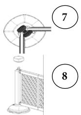
For right angle fence assembly, rotate the corner post 45 degrees before installing the next section of paneling.
